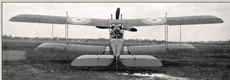
An early RAF built RE.8 (possibly A73) from the first production batch of 50 aircraft showing the clear cellophane covered 'bottom center portion of planes' and the cockade position inboard of the ailerons. On this very first production batch of RE.8s the pilot's Vickers gun was installed inside the left side of fuselage and a Bowker mount was used in place of the Scarff ring for the observer's armament. The rear of the propeller blades appear to have been painted black to improve pilot visibility.
