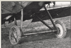
Late wooden undercarriage from rebuild RE.8 H7139. Wooden undercarriage legs were usually left unpainted with black metal brackets. Note the heavily stained starboard wheel cover, possibly from oil spilled when filling the tank immediately above.
