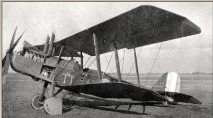
Standard Motor Co built RE.8 A4477 is fitted with a Daimler style cowl. A side cowl panel has been removed for access to the rear of the engine. No armament is fitted but the pale leather reinforcing patches for its Constantinesco synchronizing system are visible against the dark PC10 finish. Standard Motor Co decals can be seen on the wing struts.
