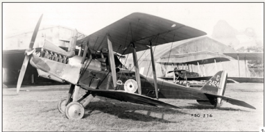
Late wooden undercarriage from rebuild RE.8 H7139. Wooden undercarriage legs were usually left unpainted with black metal brackets. Note the heavily stained starboard wheel cover, possibly from oil spilled when filling the tank immediately above.
