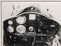
Instrument board showing one style of arranging the instruments. Note the small lamps for illuminating the instruments when night flying, RAF Mk.II compass, Very flare pistol holster and tailplane trim wheel on the right. Uncommonly the mounting brackets for the Aids sight are positioned on the left of the windscreen.
