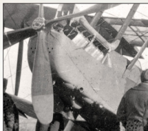
Daimler built cowl details for Brown & Barlow carburettors. Note the unpainted aluminium 'side plates' of the RAF 4A engine.
