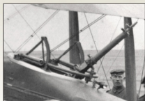
Scarff ring detail from B2293 on page 28 with a single Lewis Mk.II fitted. Note the rear facing Holt light.
