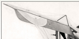
Port upper aileron detail from B2293. Note how the white border of the cockade runs up to and 'over' the rear edge of the aileron, indicating it was probably painted at a later date than the red, white and blue of the cockade.
